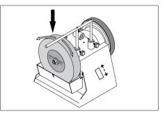
securing the tool with the tool clamp or tool holder, and setting the honing angle to the angle used when grinding the tool.
