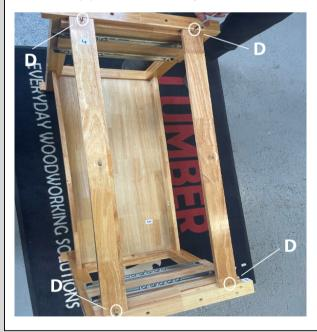
To attach the middle drawer runner (6) use screw (D) ensuring the screw locates into the pilot hole on the middle drawer runner (6) as shown in below image.
