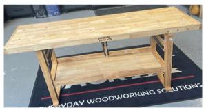
Finally, attach the vice (7) to the front of the table top (5) into the pre drilled holes on the right.
