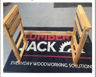
Insert bottom shelf (3) by sliding into the recess of the support bracket (2). Then attach the second support bracket (2) to the side legs (1) using bolt (C), washer (C1) & dowel nut (B)
