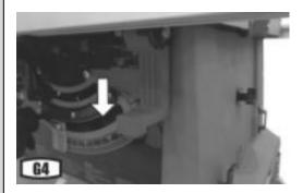
NOTE: Make sure the locking handle is locked securely.
