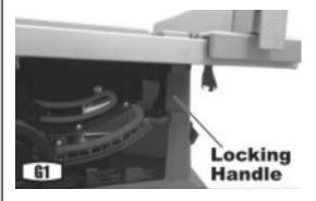
When the locking handle is in the "UPPER" position the extensions table is free to be adjusted (See Fig. G2).
