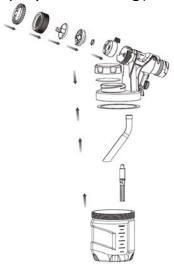
**Note:** The spray tip must be assembled in the sprayer with the bumps on the spray tip in vertical direction **Note:** Assemble the pickup tube(#15) and check valve (#16) by firmly pushing them onto the inlet on the sprayer.
