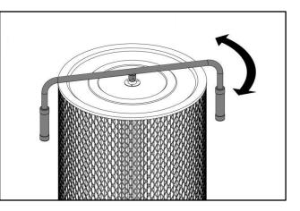
The use of compressed air or liquids to clean the canister filter will damage the filtration pleats of the filter. Use ONLY the cleaning handle or, if necessary, use a soft brush to clean the inside of the canister filter.
