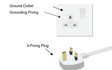
**WARNING:** Improper connection of an equipment grounding conductor can result in the risk of electrical shock. Equipment should be grounded while in use to protect operator from electrical shock.
