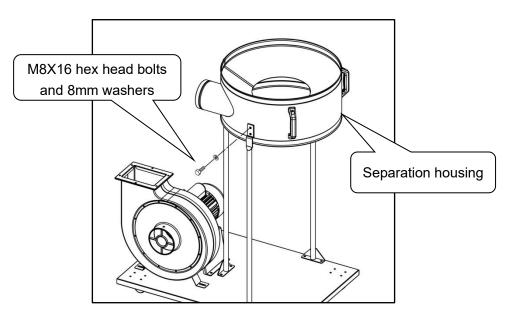
4. Attach the cleaning handle onto the shaft of canister filter, tighten hex head bolt. Install the canister filter assembly and dust bag to the upper and lower port of separation housing with the clamp.
