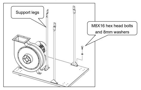
3. Install the separation housing to the three support legs with M8X16 hex head bolts and 8mm flat washers.
