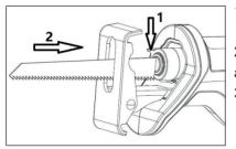
1) Open the tool holder lock and press down.
