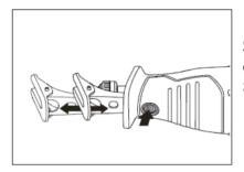
1) Press the cutting support lock down.
